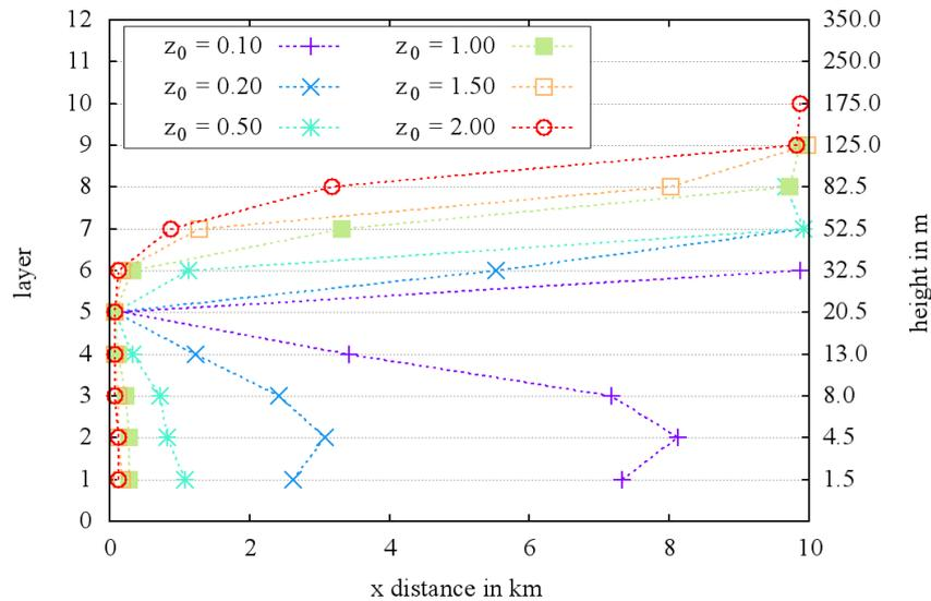
**Figure 1.** Points of maximum concentration for separate layers over the distance in x direction from the source for varying roughness lengths. The dispersion category is hold at very stable conditions for the shown roughness lengths.
